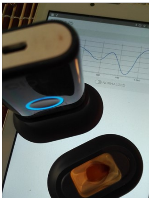
Figure 1. NIRS-SCIO™ (Consumer Physics, Tel Aviv) device ready to scan a kernel.
