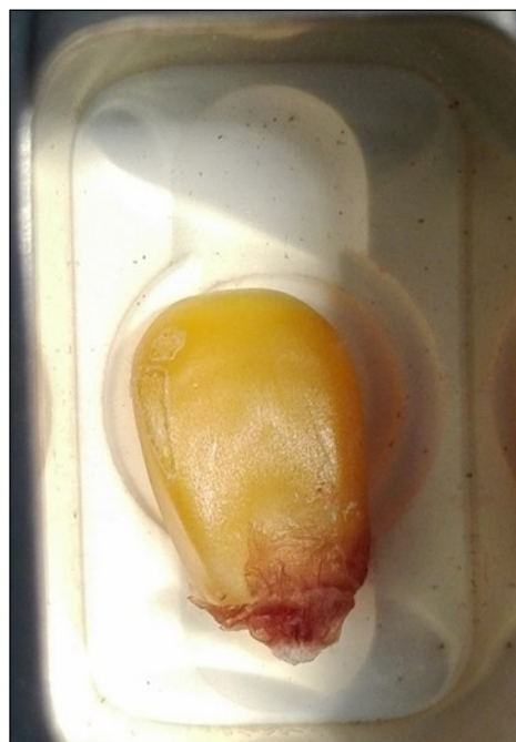
Figure 2. A kernel in the center of the reverberant pill sample holder, with the embryo facing downward.
